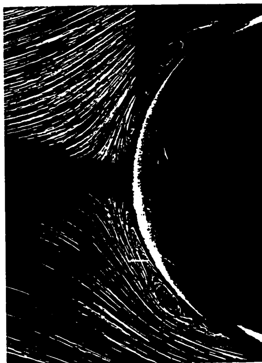
Figure 5.26: Pathlines and vorticity contours (top) and experimental result (Bouard and Contanceau, 1980) (bottom) for Re = 4750 at t = 1.5 .
